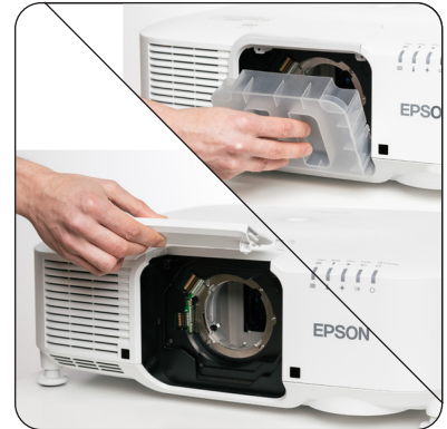
3. Place the projector on the table. Remove the lens cover and the top cover.
